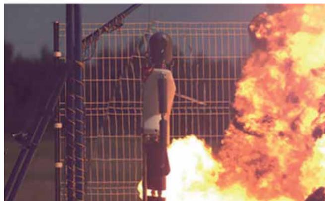
Investigating the human body vulnerability to blast waves using numerical simulation (left) and experiment (right)
