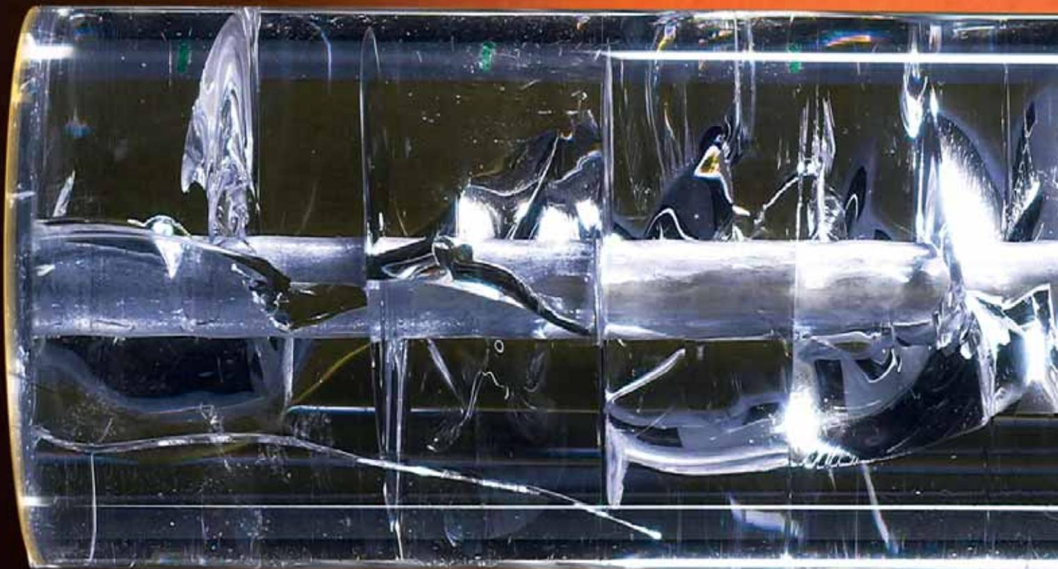
*Art and science: the effect of a solvent on a tube used for pyrotechnic tests*
