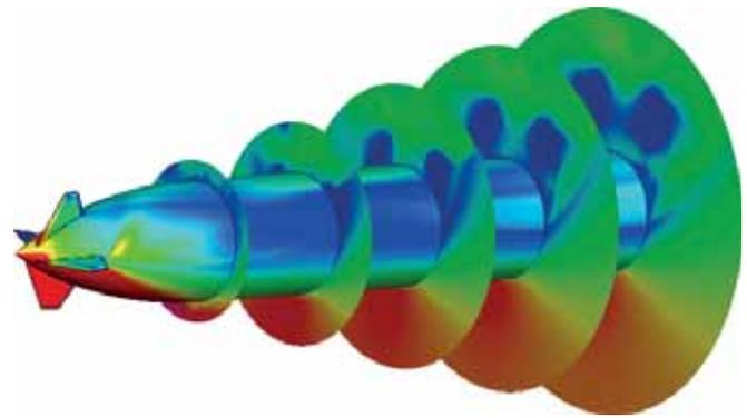
*Simulation of the flow around the decoupled fuze guided projectile*
