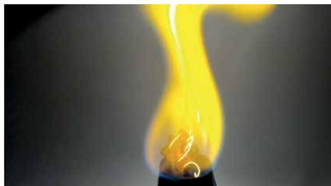
*Combustion of propellant grains*
