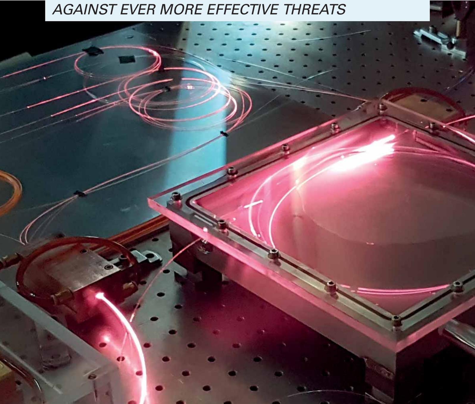
*Alignment-free all-fibred laser set-up*
