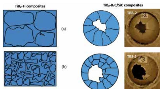
Cracks observed after impact for various samples
