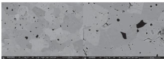
30-mm diameter (left) and 60-mm diameter (right) samples of SiC-doped  $TiB_2$
