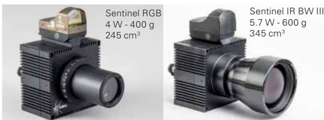
ISL's visible (left) and infrared (right) Sentinel UGS
