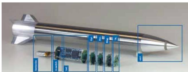
Components of an embedded navigation unit
