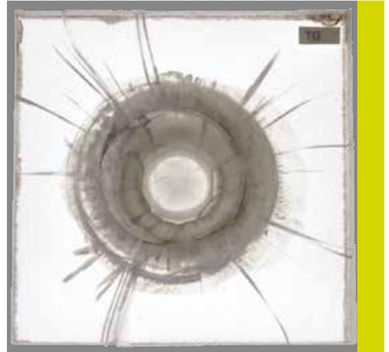
*Composite visor sample after drop tower impact*
