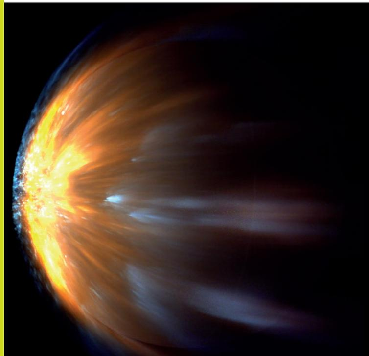
*Hypersonic flow field around sphere body in ISL shock tunnel showing influence of generated plasma on radar signature quantified*
