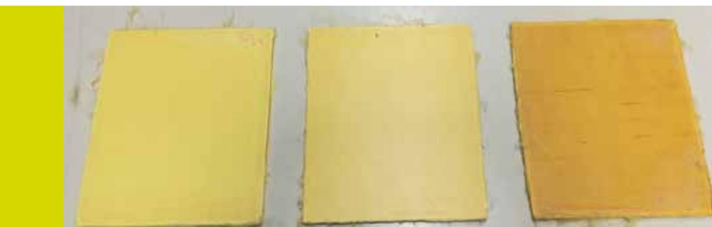
*Comparison of aramid helmet composites before (left) and after ageing using different artificial ageing cycles (centre, right)*
