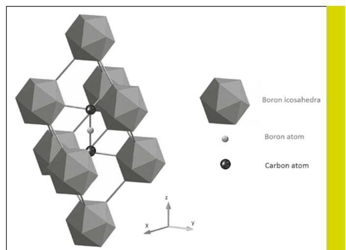
*Schematic view of the crystallographic structure of Boron Carbide ( $\text{B}_4\text{C}$ )*
