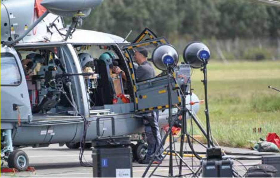
Setting up the shot noise measuring device in a helicopter cabin
