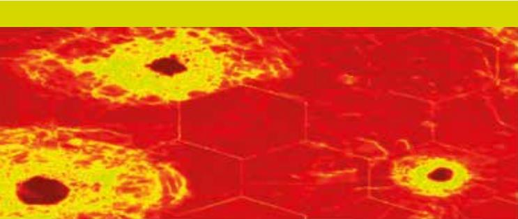
*Non-destructive testing image of protective plate after ballistic testing*
