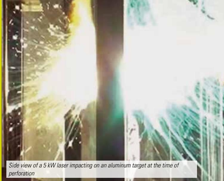
Side view of a 5 kW laser impacting on an aluminum target at the time of perforation
