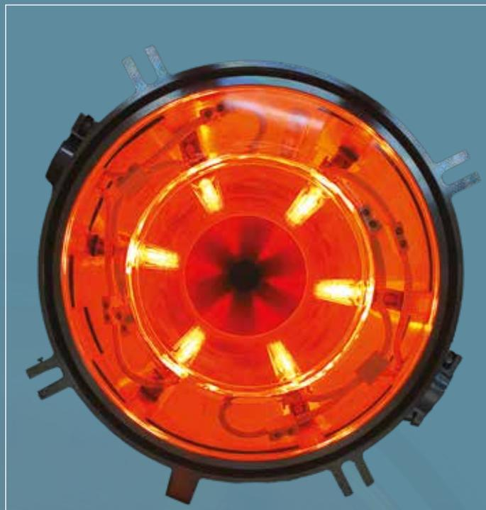
*Atomisation chamber of the spray flash synthesis (SFS) process warmed by infrared heaters*
