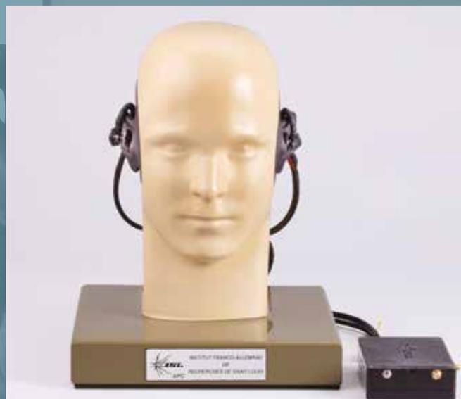
*New generation hearing protection device used in the PACOPAC project*
