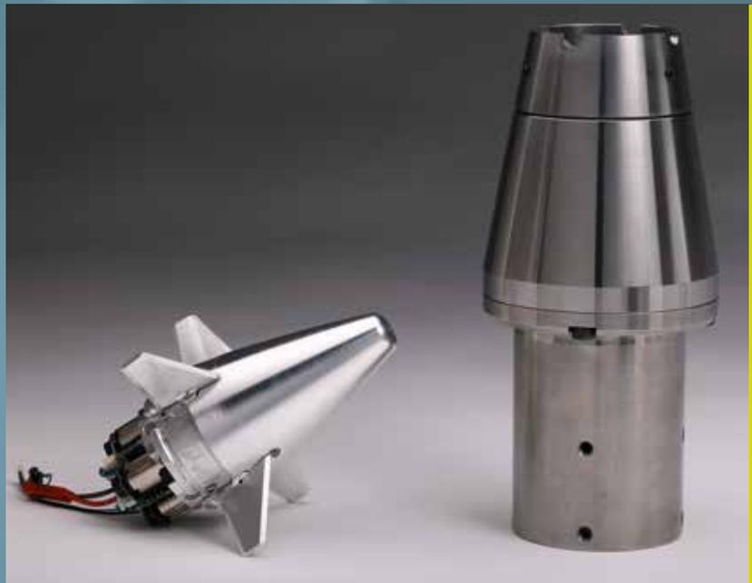
*The decoupled fuse demonstrator for use in wind tunnel at subsonic speeds
