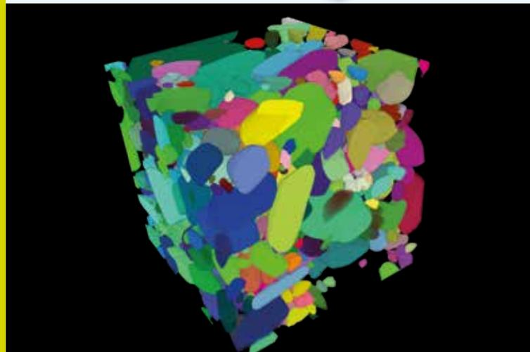
*Numerical extraction of particles of an explosive formulation
