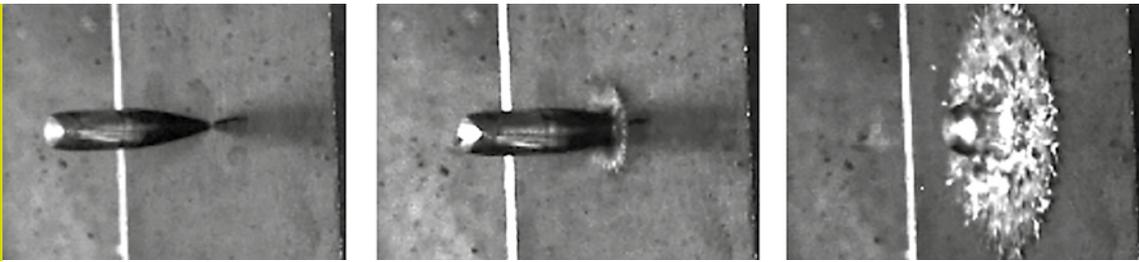
*Ceramic plate stops a hard-core bullet calibre 7.62 (frames taken by high-speed camera)*
