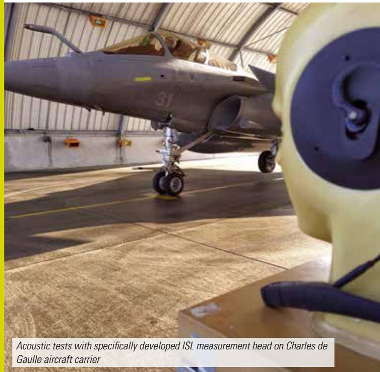
*Acoustic tests with specifically developed ISL measurement head on Charles de Gaulle aircraft carrier*
