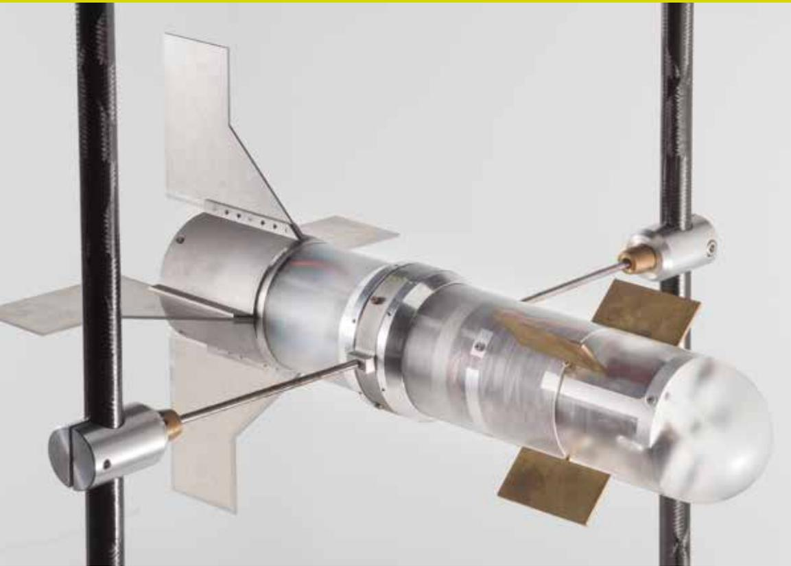
*Hardware In-the-Loop (HIL) Wind Tunnel model*
