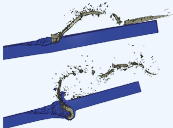
Numerical and experimental investigations on ricochet at impact velocity of 1400m/s against homogeneous armour
